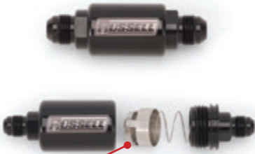
Piston-face o-ring seal for positive sealing to prevent flow back
